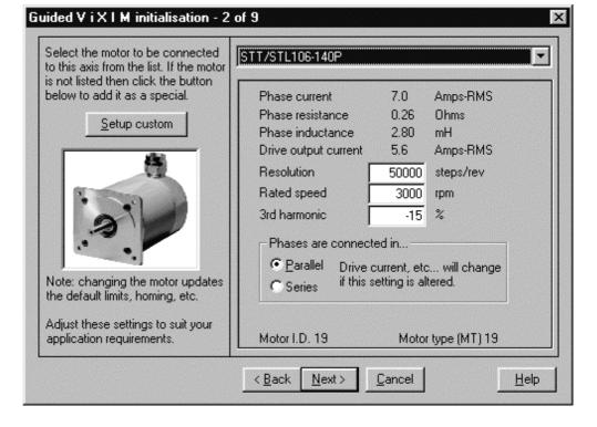
Press 'Next' to select Motor Standby current and In-position settling Time values.
